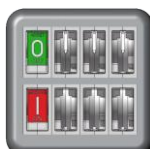
COUPURE VISIBLE VISIBLE BREAKING
